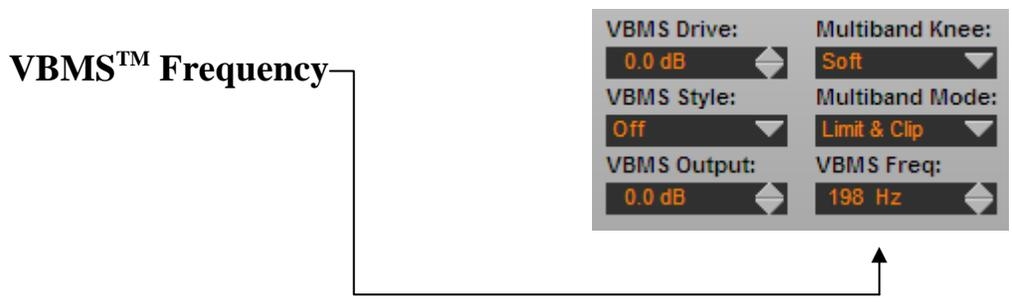
The VBMS™ Frequency is adjustable over the range of 60Hz to 300Hz with audio information that is present below the Frequency setting being processed by the algorithm.
