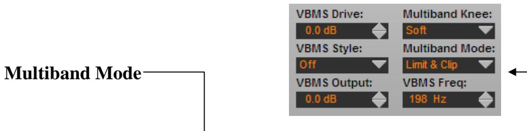
The Multiband Mode control is present *only* on the AP1000 product and selects one of four different operating modes for the 31 band limiter and its associated 31 band distortion masked clipper.
