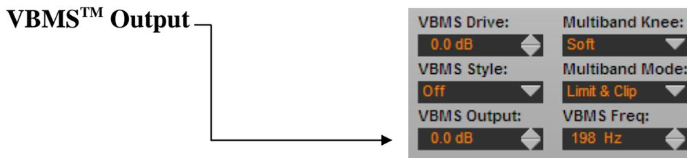
There are no particular cautions associated with adjusting the VBMS™ Output and Drive controls other than some care should be exercised when setting the Output control higher than approximately +3dB *when* the Drive is *also* set higher than approximately -2.0dB. This is because under those conditions certain program material *might* cause sporadic unmasking of spectra that the algorithm is charged with keeping hidden below the masking threshold of its adjacent critical bands.
