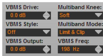
The Drive control adjusts the relative position of the 3dB-wide operating window within the available dynamic range exiting the five band AGC/Compressor and is adjustable over a +/- 10dB range.
