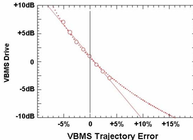
If it were possible, theoretically perfect behavior would be represented by the vertical line extending above the “0” on the horizontal axis.
